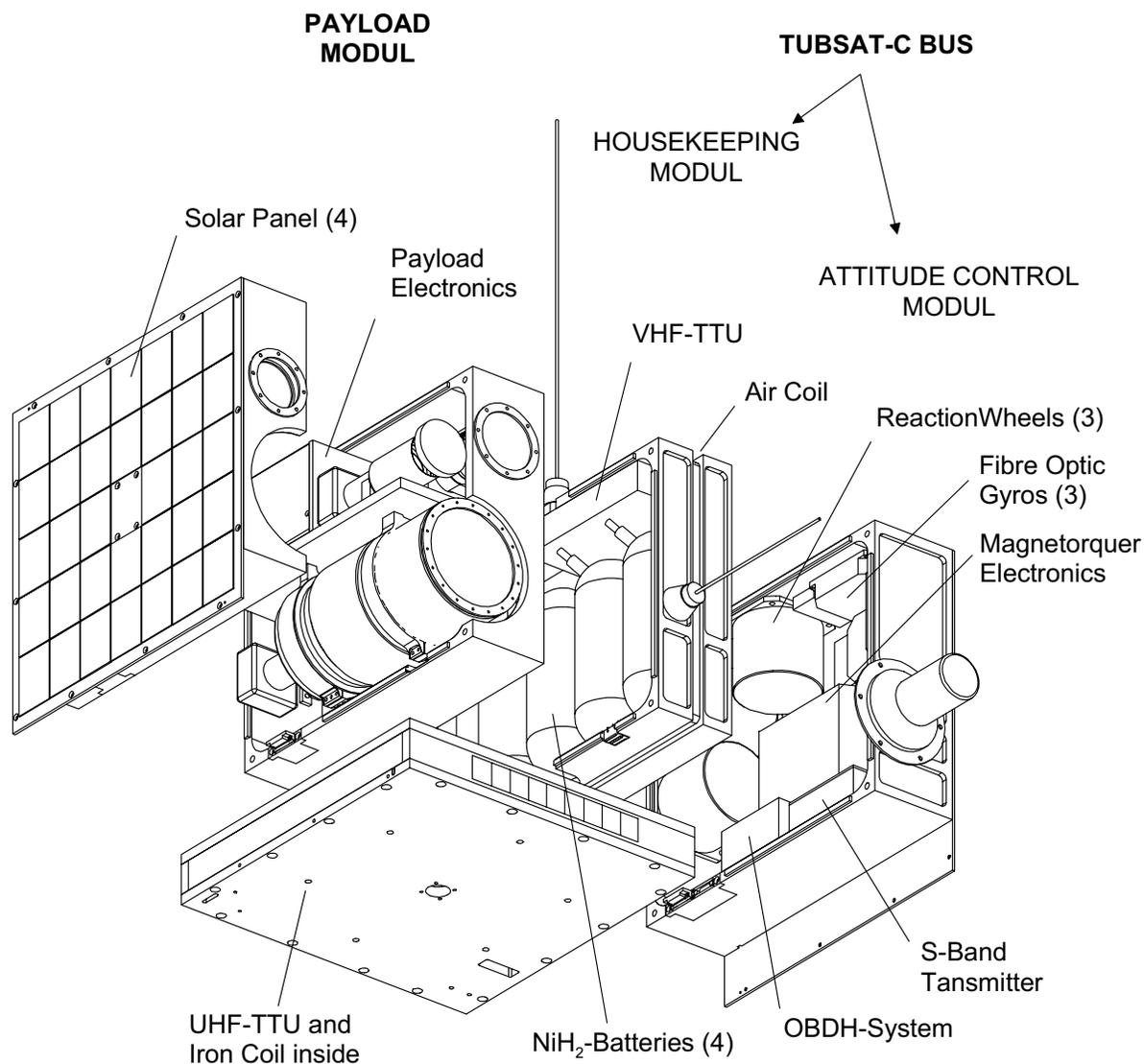
**Figure 3:** Exploded view of the microsatellite DLR-TUBSAT
