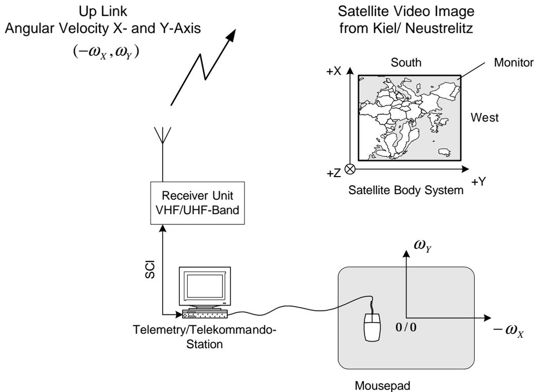
**Figure 7:** Mouse Control Station at TUB
