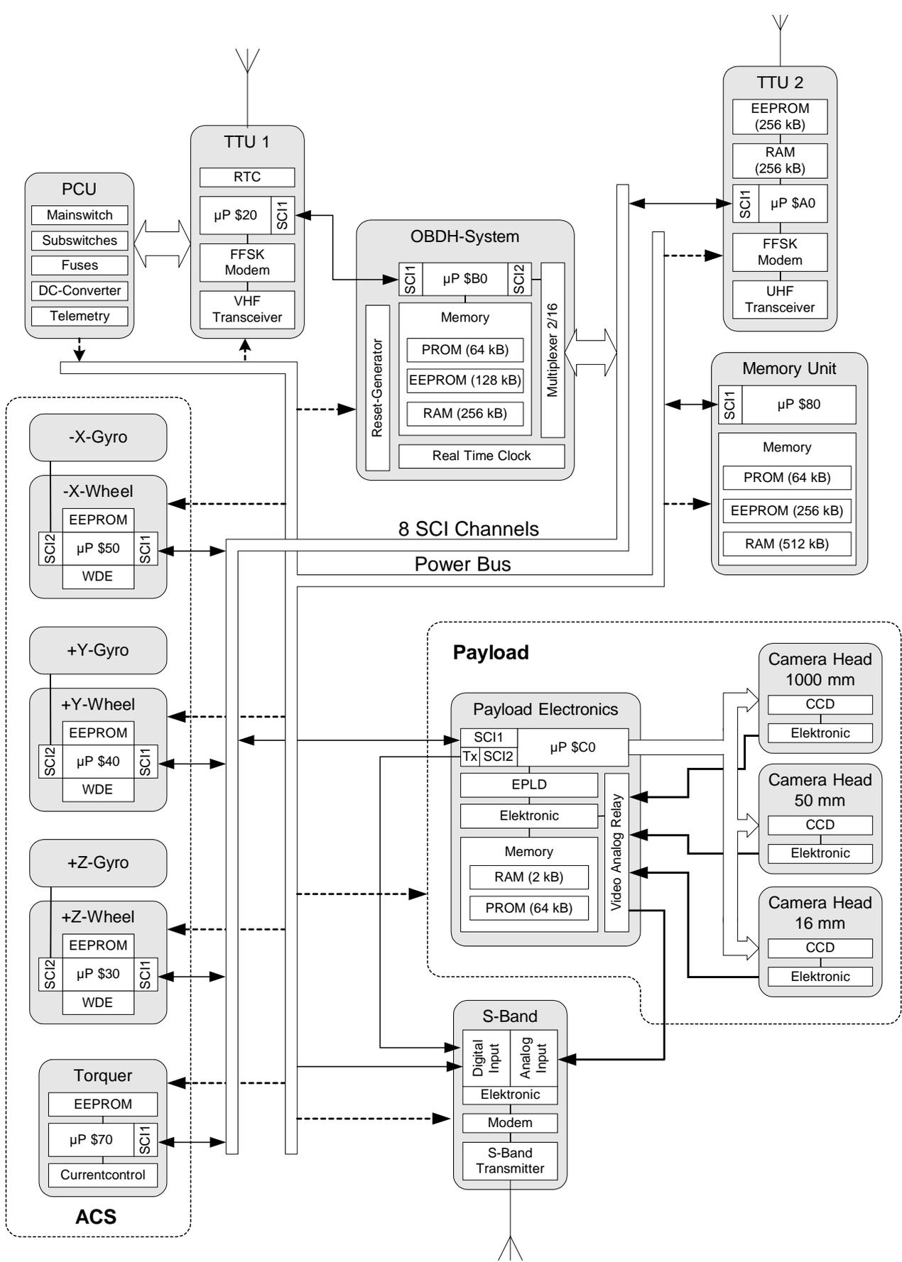
Figure 4: System architecture of DLR-TUBSAT
